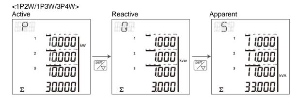
•Eco-POWER METER displays the power as below.
