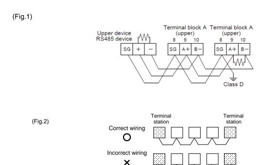
♦How to connect KW9M and the other devices with 2-wire system
